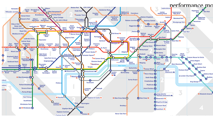
Fig.1. An example of the classic octilinear schematic representation used in most metro maps today and originally developed for the London Underground map by Harry Beck in 1931.
