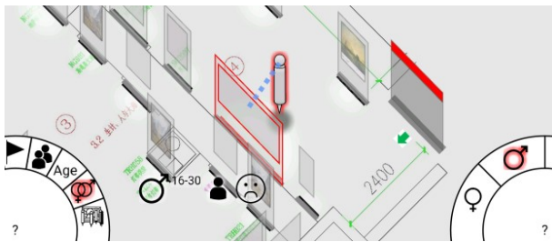
Figure 4: The tracking application interface. The user presses on different exhibits to indicate the movement of a visitor and uses the thumbwheel dials to specify visitor characteristics or actions.
